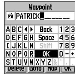
An example of data entry with ‘OK’ selected. Use the ‘OK’ selection to complete data entry.
